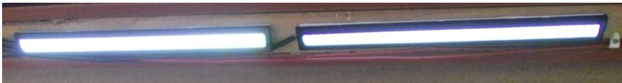
The Load side of the controller I connected to my lighting circuit. Again, looking to reduce noise I went for LED's, bright, low current, low voltage, ideal for my needs. I picked up two sets of LED strips used on cars. These were light weight very bright, thin and above all very cheap (Just over £3.00 a set).
