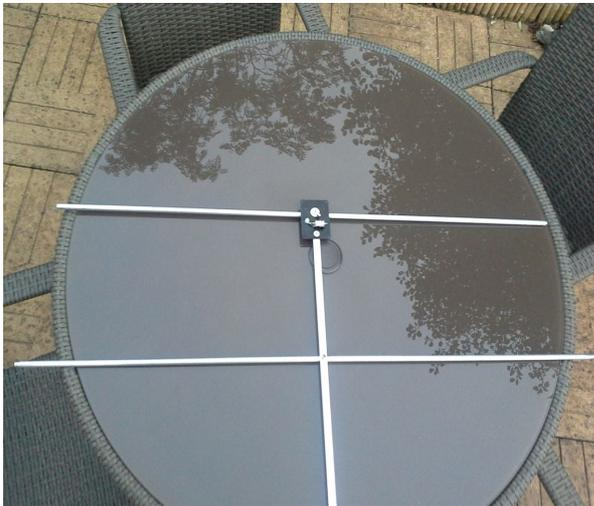
*Illustration 4: HB9CV assembled elements and boom with tuning capacitor*
