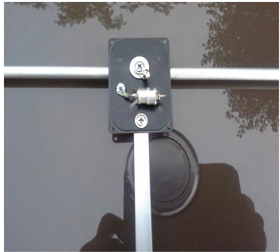
*Illustration 5: HB9CV Tuning capacitor detail*
