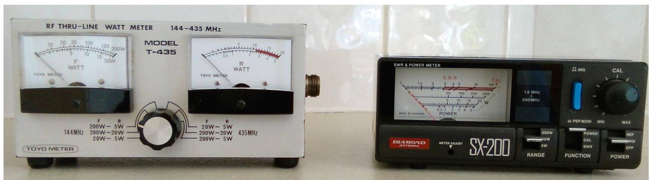
Illustration 1: Pictured Left a Thru-Line Watt Meter and Right an SWR Meter
