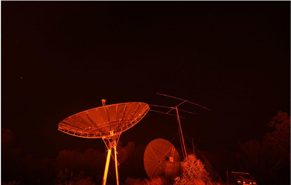
ANZAC Field Day – dishes for 23 cms one for Earth-Moon-Earth and a dish in the background for terrestrial DX, plus the TH-3 HF antenna.
