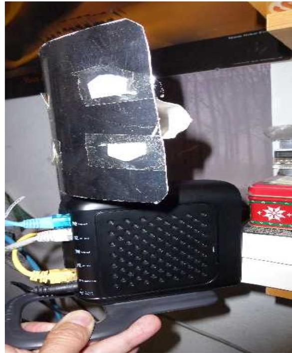
The parabolic reflector will need to be covered in aluminium foil. I used the cardboard for my reflector and glued kitchen foil to it. I also cut longer tabs for the former/spacer part of the aerial. It does not matter which side of the reflector you glue the foil to. However, if the foil is bent one way it may crinkle slightly and bent the other way it may stretch. I went for stretch. Go ahead and try the reflector out.
